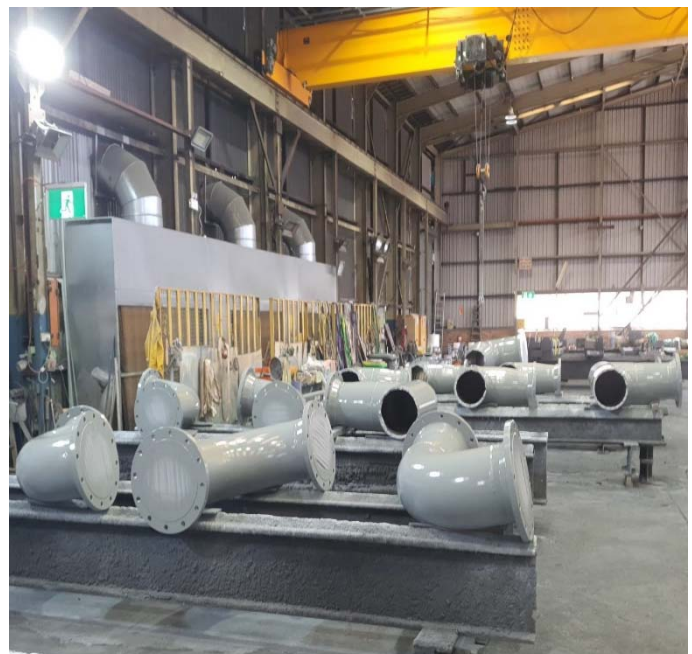
Top Coating of Pipe Spools
