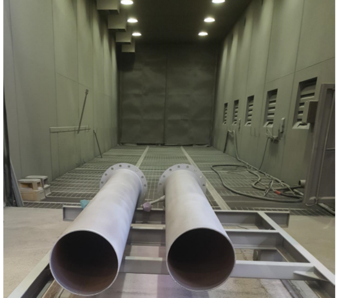
Blasting of Pipe Spools
