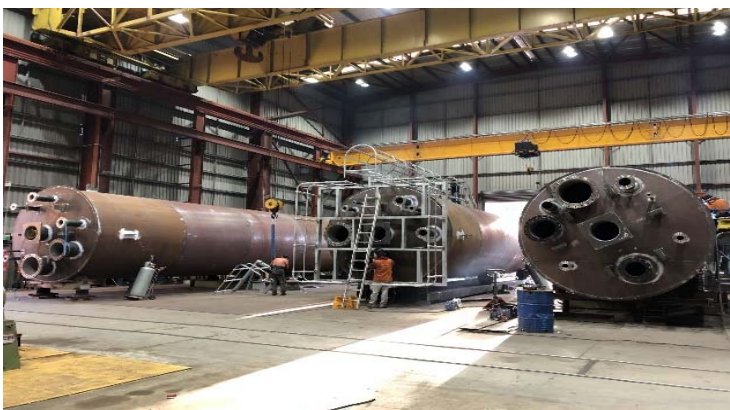
50t & 100t Vertical Bitumen Storage Tanks
