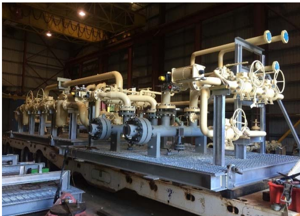
Gas Piping Skid
