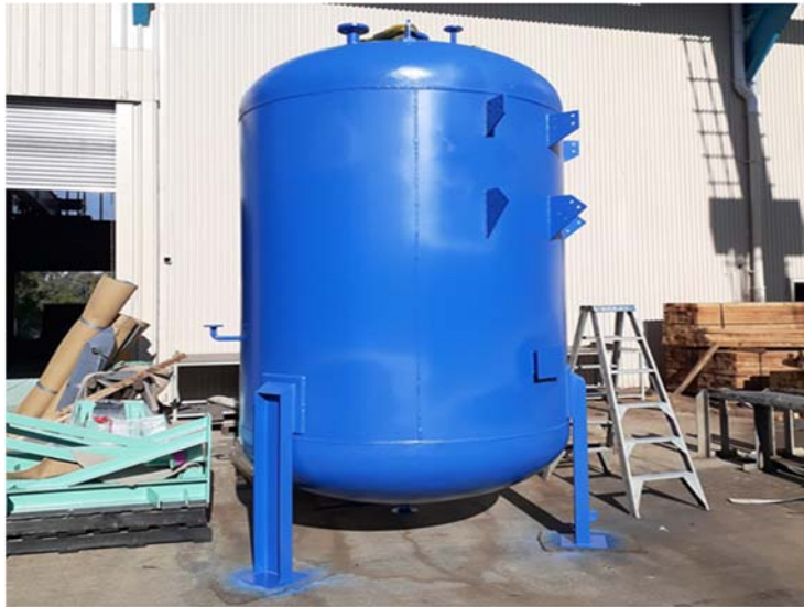
Vertical Pressure Vessel
